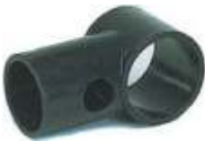
Steering Joint - acts as a 360 degree pivot - standard tube fits through large hole - standard connector end fits into small arm - used for steering shafts - not the same as the 1-hole coupling
